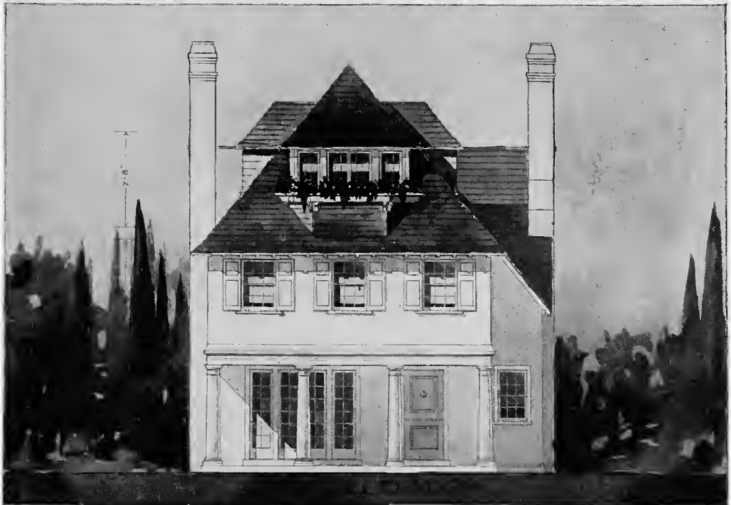
Front and side elevations of Design No. 10. Shingles or clapboards might be substituted for the stucco walls, resulting, in most localities, in a saving in the cost
